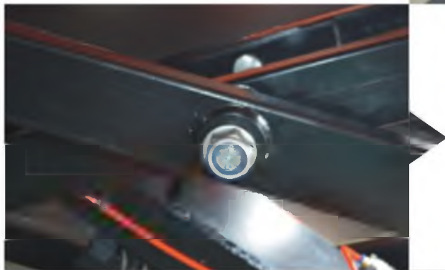
活动关节都装有自润轴承 Joints with self-lubrication bushing
